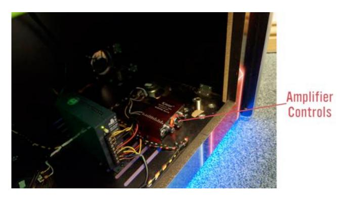
The amplifier controls can be just inside of the machine as seen above. The large central dial changes the volume, and the smaller dials will alter the bass and treble respectively. The amplifier can be switched off completely using the push-button the left of the dials.
